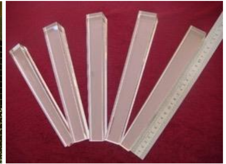
24cm-long BGO crystals for LEP L3 experiment (CERN, 11,000 kg)
