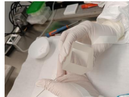
^{100}\text{Mo} enriched LMO crystals ( 45 \times 45 \times 45 \text{mm}^3 ) developed in SIC
