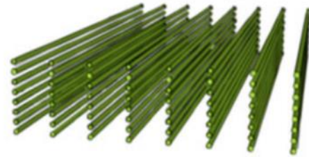
Layers of Crystal Fibers in a sampling calorimeter
