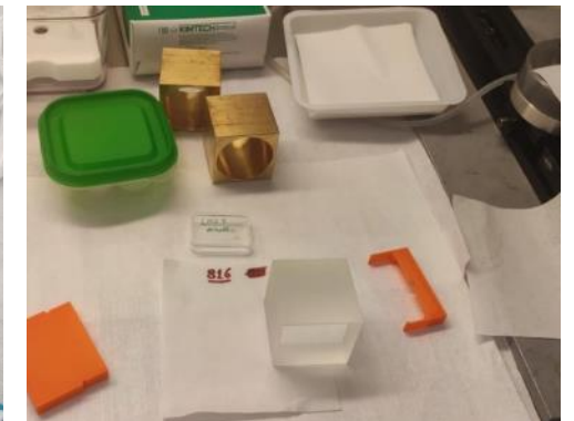
^{100}\text{Mo} enriched LMO crystals ( 45 \times 45 \times 45 \text{mm}^3 ) developed in SIC
