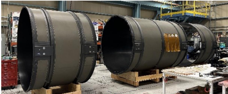
Global Structure :Outer Cylinder (OC) Hosts the ITk
