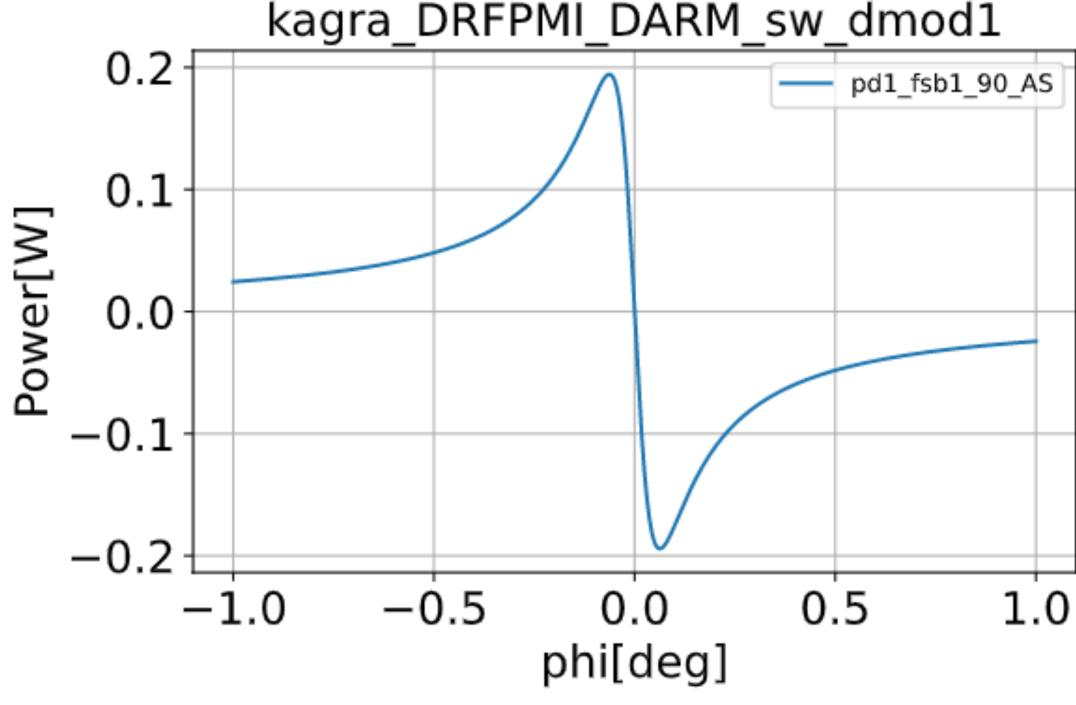
Demodulation frequency is 16.881 MHz and demodulation phases is **Qphase**.
