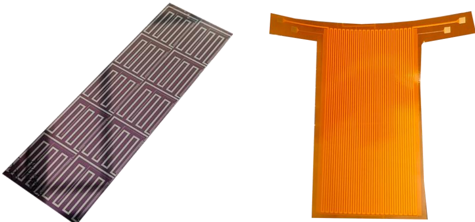
Realistic thermal dummies for cooling tests produced for barrels (left; silicon) and disks (right; FPC), with dedicated regions for matrix and peripheral power dissipation.
