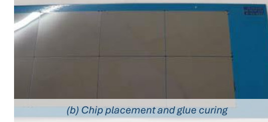
Module assembly procedure with dummy components by using MEMPACK multi-purpose machine die bonder.
