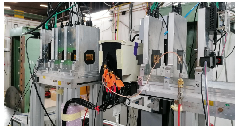
DUT mounted on a 16-ch analog board
