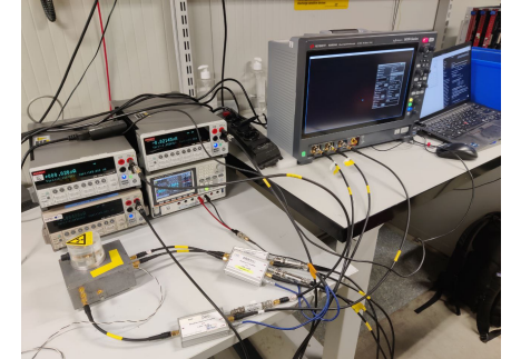
Interim ^{90}\text{Sr} setup (Source from the CMS ETL System Test group)
