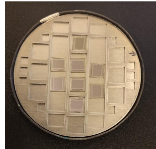
Setup for gamma irradiations of MAIN sensors and minis
