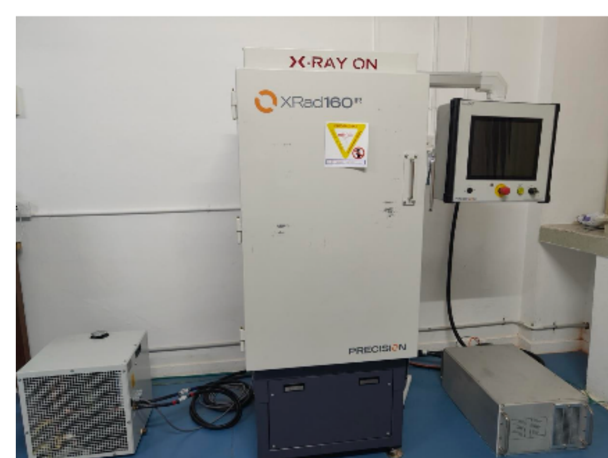
X-ray irradiator: Use tungsten target, capable of generating x-rays upto 160 kVp.
