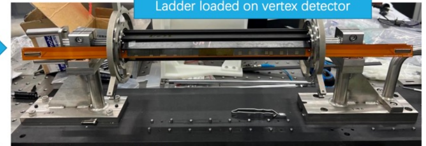
Ladder loaded on vertex detector
