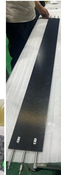
Prototype stave support CFRP faces + CF honeycomb, Ti cooling tubes
