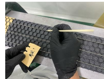
Prototype stave support CFRP faces + CF honeycomb, Ti cooling tubes
