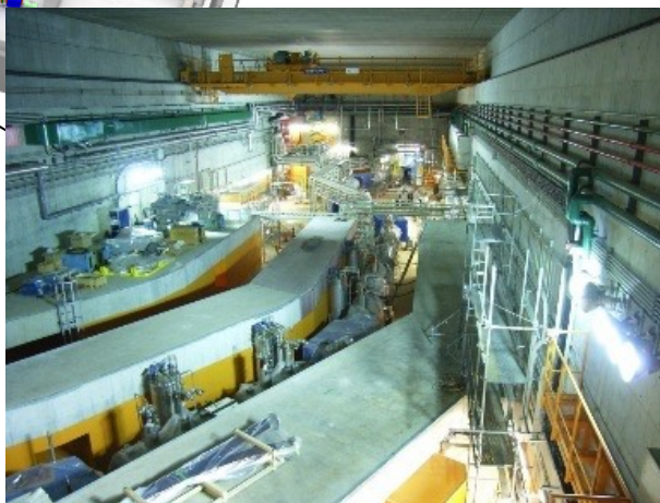
BigRIPS: Superconducting RI beam Separator In-flight separator World's Largest Acceptance High magnetic rigidity 9 Tm
