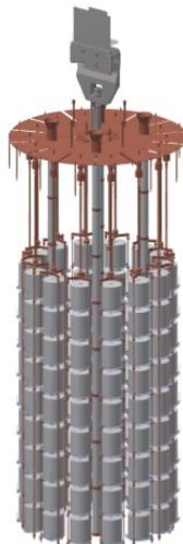
New String layout, PEN det. plates, front end electronics, & DAQ
