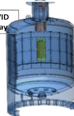
Upgrade GERDA cryostat: new lock, cabling detector suspension
