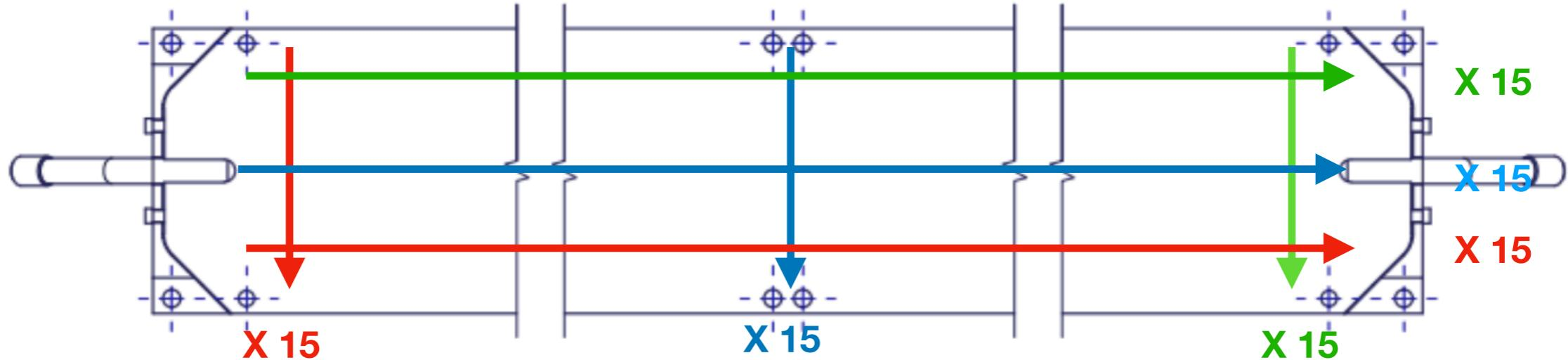
Transverse / Longitudinal directions : 45 measurements
