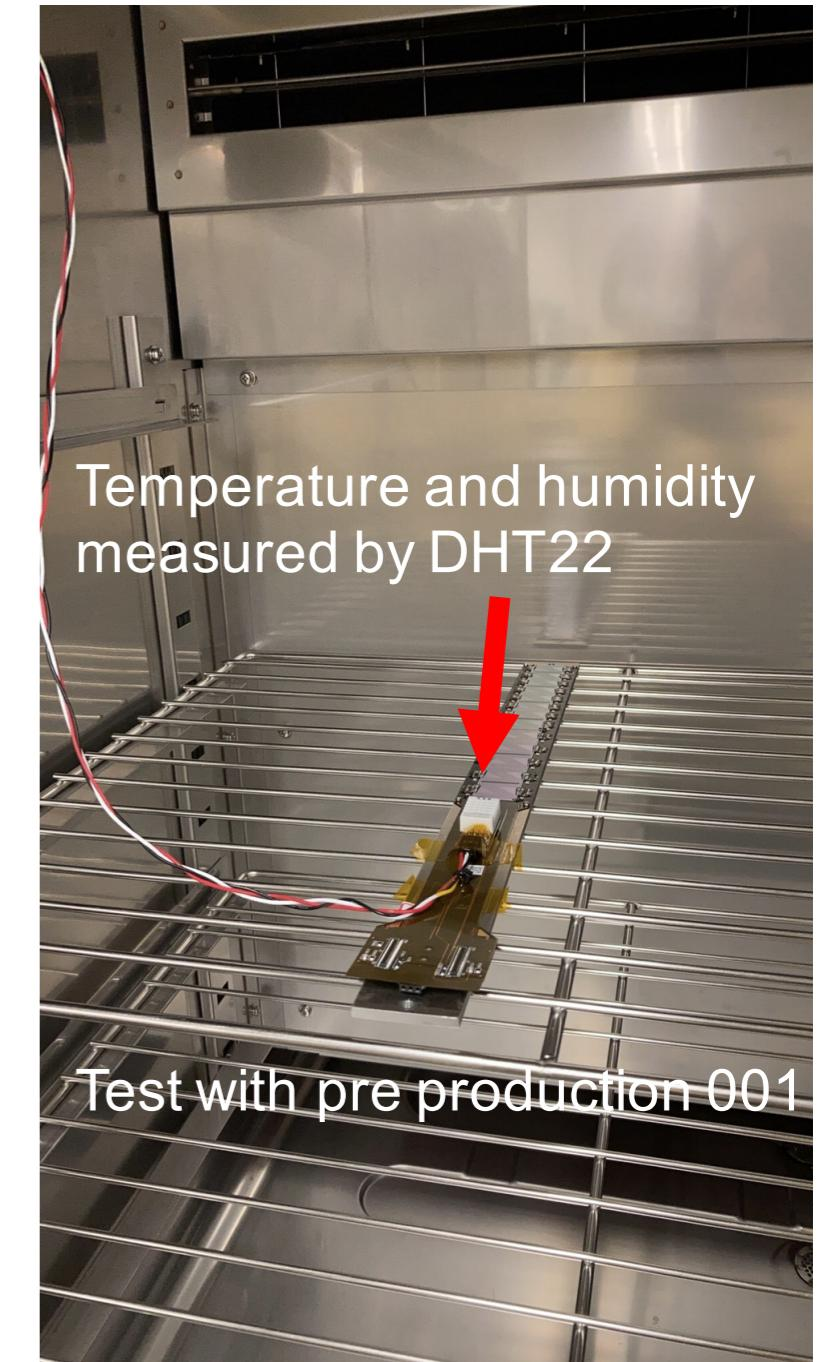
The calibration test result after thermal cycle is consistent with the case before thermal cycling
