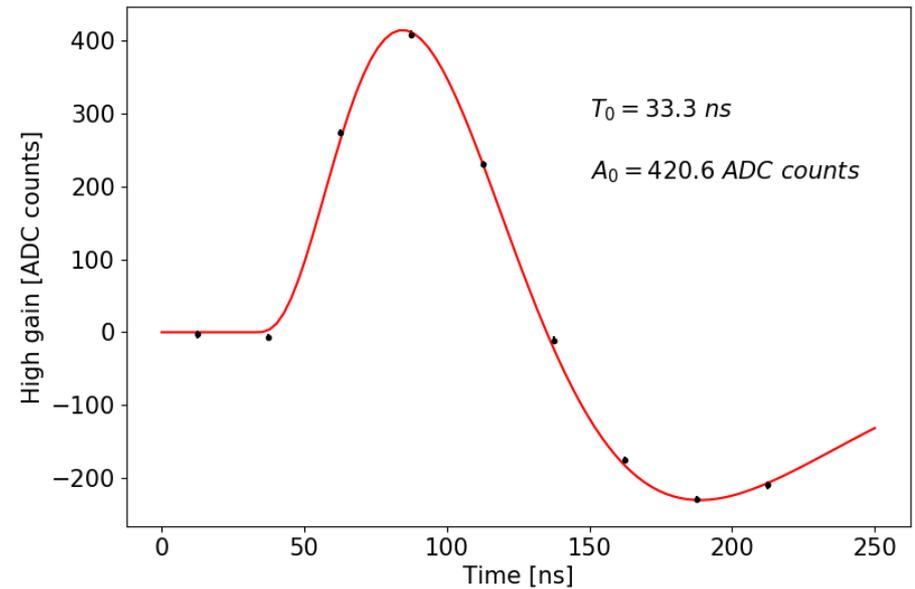
Low gain shaper pulse (left) vs High Gain pulse (right) for 300GeV electrons.
