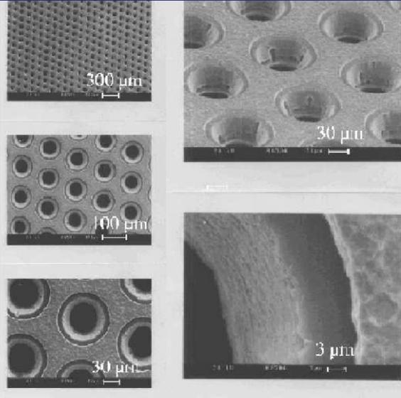
Thin perforated kapton foil, metal clad on both sides. ( $\sim 500\text{V}$ )
