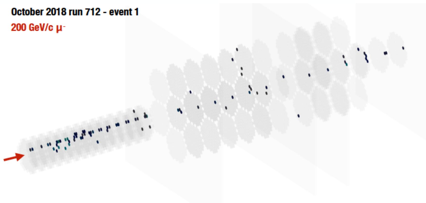
**Figure:** Event display of a 200 GeV/c muon traversing the CE-E (28 layers) and CE-H (12 layers) prototypes during the beam test of October 2018. The incoming muon enters the detector from the left-hand side.
