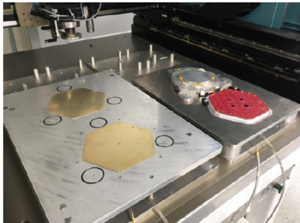
*8 inch HGCal Silicon module assembly set-up
