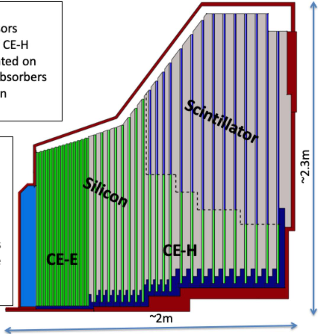
Electromagnetic calorimeter (CE-E): **Si**, Cu & CuW & Pb absorbers, 28 layers,  $25 X_0$  &  $\sim 1.3\lambda$
