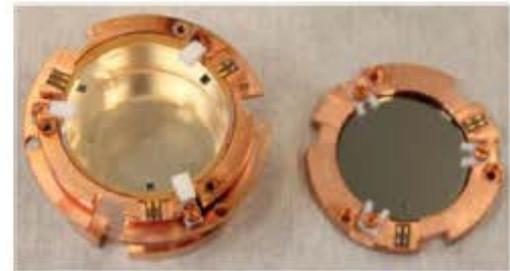
Detector module for CUORE (top) and CUPID-Mo (bottom) with NTD-Ge – 5 -7 keV FWHM
