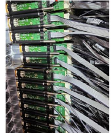
Photomultipliers (PMTs) and HV divider base
