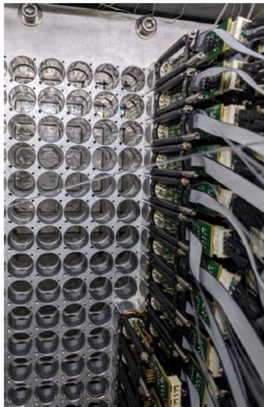
Divider base boards were removed for bypassing
