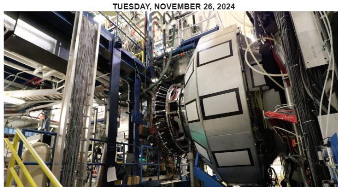
A view of the Central Neutron Detector in Hall B's CEBAF Large Acceptance Spectrometer for 12 GeV (CLAS12).
