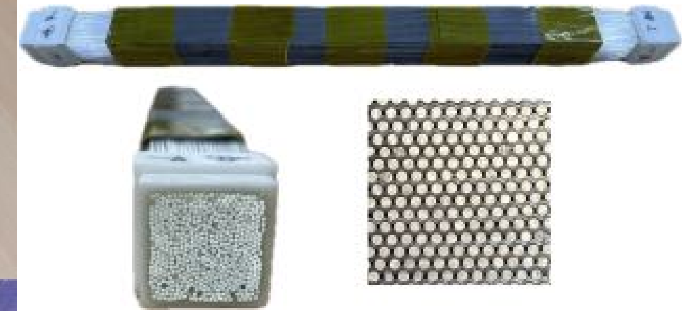
scintillating-fiber stacking 3x3x32 cm 3 prototype module
