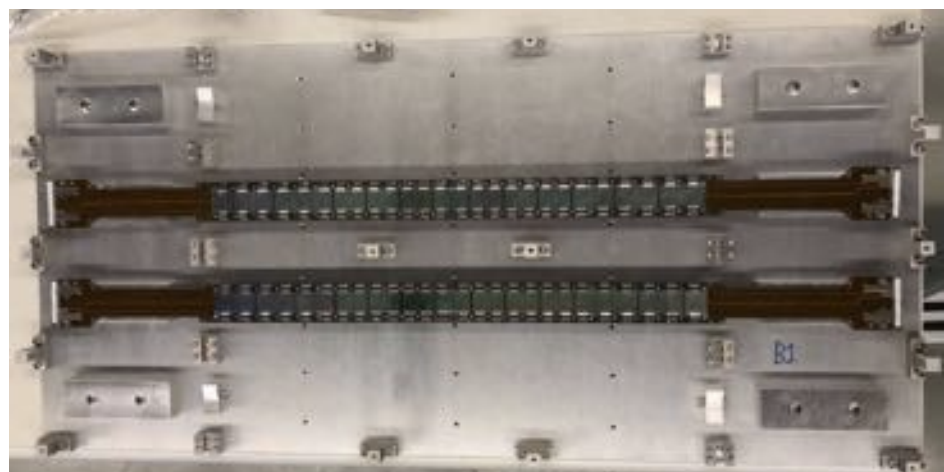
Assembly of INTT ladders
