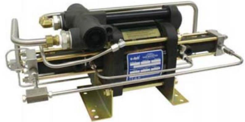
High-pressure booster (Haskel 86981) Inlet: 17 bar Outlet: 1034 bar/15000 psi
